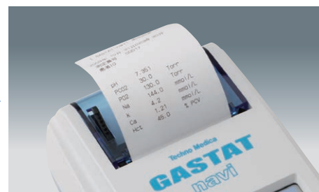
STEP 3 Test result is printed and appeared on the display in 45 seconds. ANALYZE
