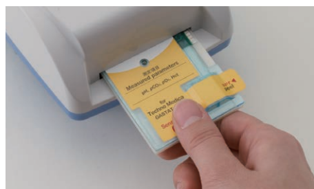
STEP 1 Insert a sensor card. INSERT
