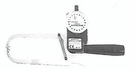
The Harpenden Skinfold Caliper is a precision instrument designed for use in the performance of skinfold thickness measurements (from which estimates of body fat are derived). The use of this instrument has been well established and documented over the past 40 years.
