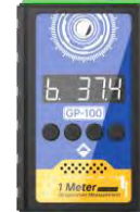
Default alarm threshold is 37.4°C
