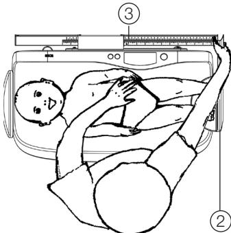
2. Using your right hand, push the foot support (2) in the direction of the baby's feet, placing the baby's feet on the bearing surface of the foot support. Keep the baby still on the weighing tray with the left hand.
