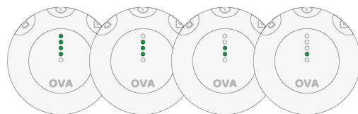
When battery is 20% and 10%, a low battery alert will play and all white LEDs that are active will flash.
