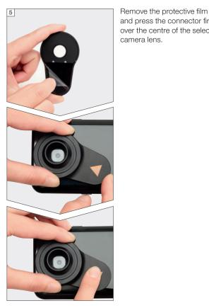
and press the connector firmly over the centre of the selected camera lens.
