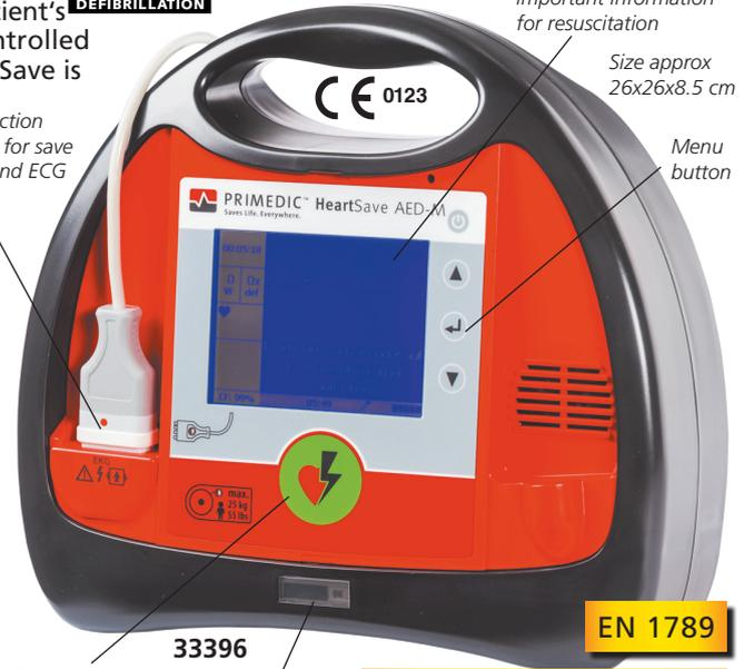
Connection socket for save pads and ECG cable
