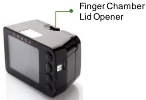
3. While holding the TensorTip with your right hand, insert the index, middle or ring finger (depending on which fits best) of your left hand with the bottom side of your finger in contact with the Chamber floor and touching the front of the Chamber. The fingertip should not be pushing the front of the chamber and should completely cover the Chamber Lens.
