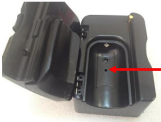
Insert a pin gently into the hole on the chamber base to reset the hardware.
