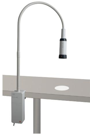
The EL10 LED examination light distinguishes itself through an absolutely homogeneous field of light. The light intensity can be regulated continuously between 6,500 and 45,000 Lux. The spot size can be adjusted in a diameter between 8.5 and 14 cm to suit any situation. Both at a working distance of 30 cm.
