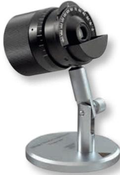
This model eye is ideal for teaching and practice. The pupil diameter and refractive error can be set exactly and are therefore reproducible. The front lens compartment holder accepts up to two trial lenses. The cylinder can be read from the graduated scale.
