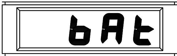
When the battery has completely expired the above will be displayed continuously and the battery must be replaced.
