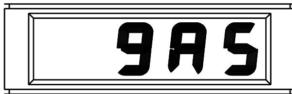
If this is displayed then turn the unit off, remove the mouthpiece adapter, and expose to ambient air for 2 minutes before repeating the test.
