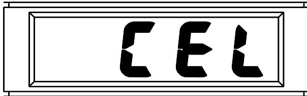
The most likely cause for this is an expired cell but may also be caused by depressing the calibration switch with no gas applied. Ensure that the concentration of calibration gas is correct (20ppm), that the connections to the gas cylinder are secure, and that the gas cylinder is not empty, and then repeat the calibration procedure.
