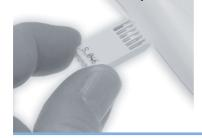
Slide the new code chip into the code chip slot until it snaps into place.
