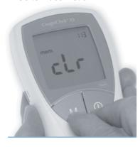
With the meter powered off, press **and hold down** the M button W. While you are holding down the M button, press the ON-OFF button and then hold down both buttons for at least 5 seconds.
