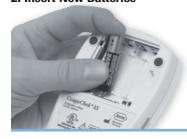
Position the batteries according to the diagram inside the battery compartment. Replace the cover. Turn the meter back over.
