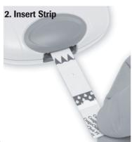
Slide the test strip into the test strip guide in the direction of the arrows until it stops.
