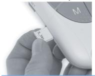
With the meter powered off, remove the old code chip and throw it away.
