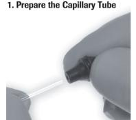
Firmly insert the end of the capillary tube into the capillary bulb. Completely insert the tube into the bulb to break the bulb diaphragm.
