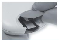
With the meter powered off, use your thumbnail to open the cover of the test strip guide by pressing its front edge upward. Move the cover safely away from the meter. Then rinse the cover with water or wipe it clean.
