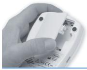
With the meter powered off, turn it over. Press the latch gently inward and lift the cover. Remove the old batteries, if necessary.
