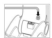
**Connecting the Connector and Plug for the Cuff** (Sold separately) 1. Insert the air hose socket into the cuff connector. 2. Insert the air hose plug to the air hose of the cuff. Air hose plug Air hose (cuff) 3. Connect the air hose plug of the cuff to Air hose plug the air hose socket of the main body. (cuff) Air hose socket (main body) Securely connect by turning the air hose plug the direction of the arrow. ☐ Use the specified connector. (Refer to page 17)
