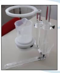
Maximum flow rate of the transducer 1 Liter. The flow transducer has some special features, such as digital calibration that can 'run the operator without having to consult an expert, weight control in real time to always have the
