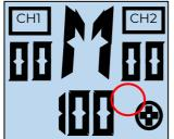
c. Press <del>CH1+ or CH1- to adjus</del>t the setting. You can select a frequency from 2 to 150 Hz.
