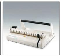
Sealing machine Termoseal: Ergonomic design and fast sealing times. Concealed roll-holder Stretched 12mm seal Dimensions: 480x198x385 mm (LXHXD) Voltage: 230V - 50/60 Hz Power adsorbed 100 W Weight: 9 kg
