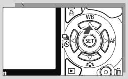
Please select the custom WB with the set-button and confirm the chosen picture with the set-button. We recommend naming the white balance picture taken with the DELTA® 20 Plus/DELTA® 20 accordingly.
